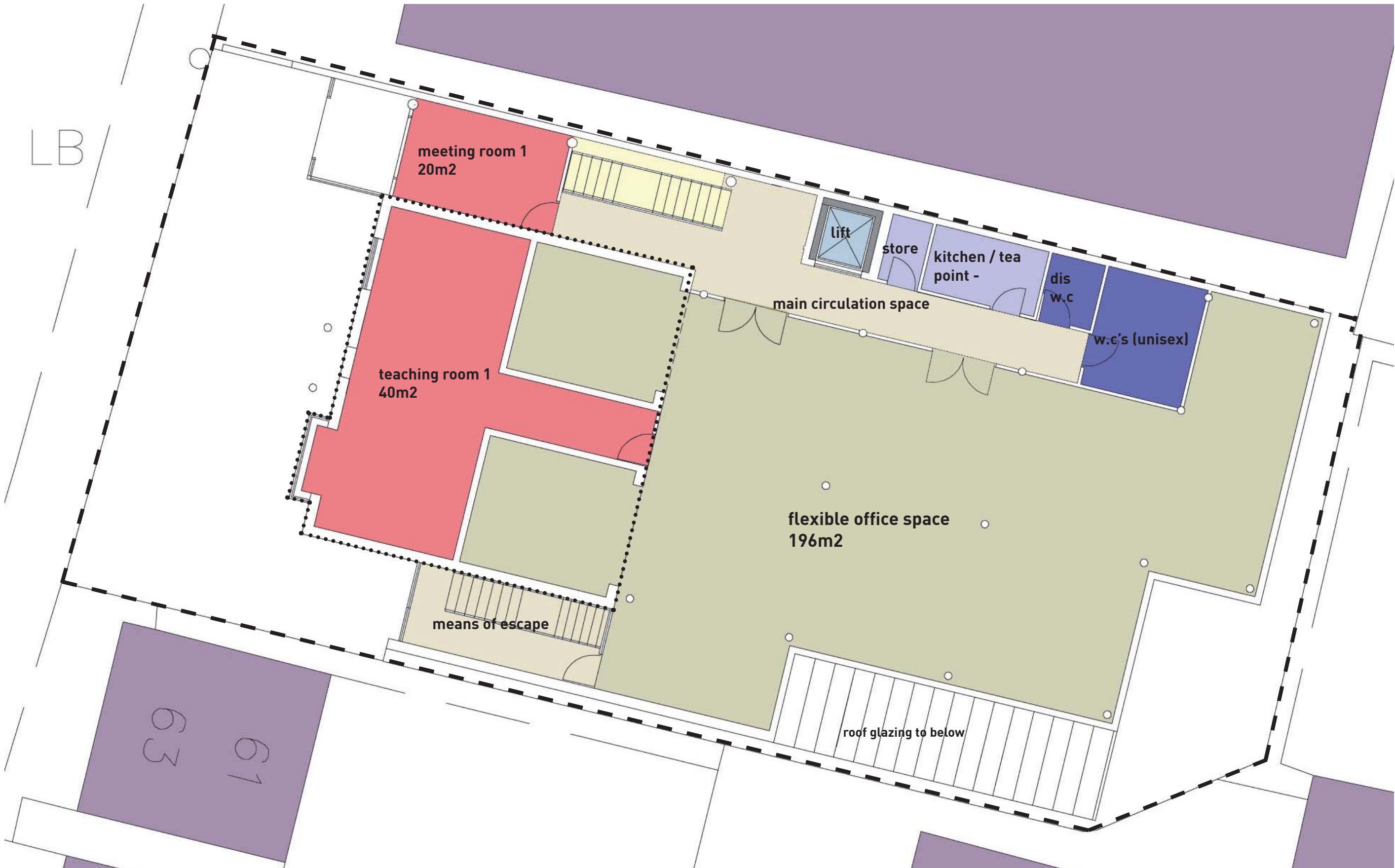
Development of 29 Church Street, Slough - Proposed First Floor Plan - Phase 2
